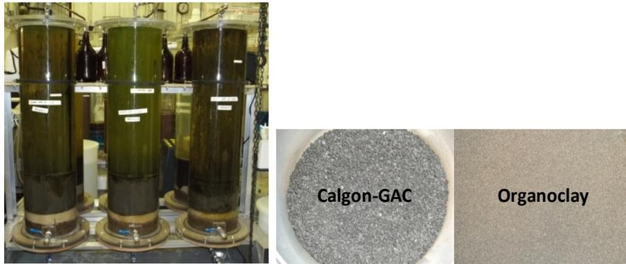
Figure 1. Column setup and amendments used for batch studies
